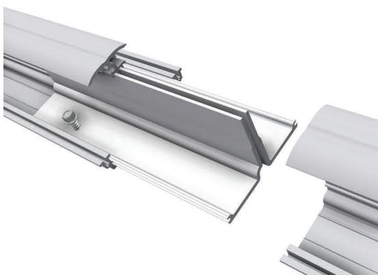
In case the length of the horizontal profile is not sufficient further profiles can be connected via the horizontal joiner. The horizontal joiners are inserted equally into the horizontal profiles and are secured against slipping by means of drilling screw.
