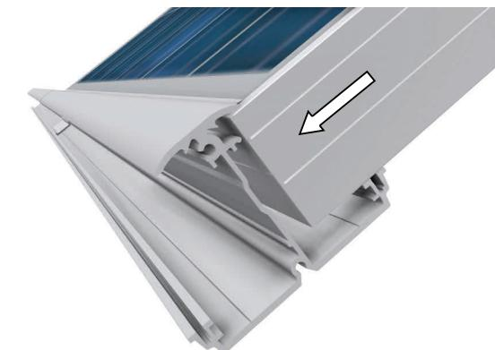
Finally the module is pulled into the profile up to the limit stop. Attention has to be paid that the module is surrounded equally from the upper and lower horizontal profile (above and below 7 mm) (compare system sketches)
