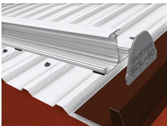
On both sides of the total profile a horizontal end cap is pushed into the plug-in channels which are foreseen in this case. The horizontal profile has to be sloped over the entire length so that on each side an air gap of about 5 mm arises.
