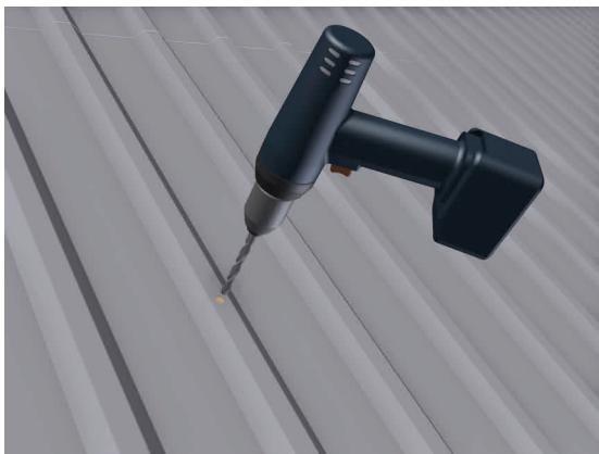
The fastening of the roof construction is done with a "solar fastener with calotte".
