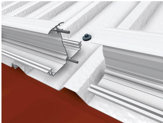
The horizontal profiles are connected via connecting pins in the plug-in channel of the profile so that the generator width results. Between the profiles there should always be a distance of 1 - 2 mm in order to compensate temperature-affected linear expansions. The horizontal profiles are delivered in 2 m lengths. If needed they can be cut with a chop saw.
