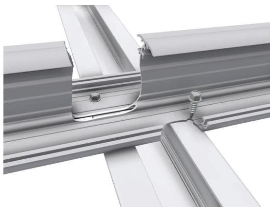
The fastening of the horizontal profiles is made via two drilling screws per junction which are bolt diagonally into the upper supporting surface of the vertical profile. The horizontal profile must be pre-drilled with 6,0 mm.
