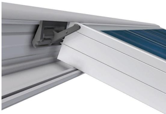
Before installing the next module insert the module protection. The **SOL-Guard** Anti-theft Protection is placed between two modules respectively and will be clipped into the upper screw duct . After having inserted SOL-Guard pull it up to the safety lever behind the first module.
