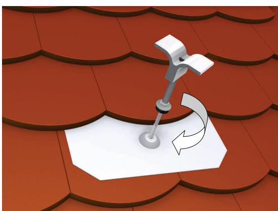
The correct position is pre-marked by the rise in the form of punched sheet metal on the roof tiles. The same applies to the pre-drilled rafters. Then the solar fastener is bolted. The mold sheet may possibly be adapted to the contour of the roof covering.
