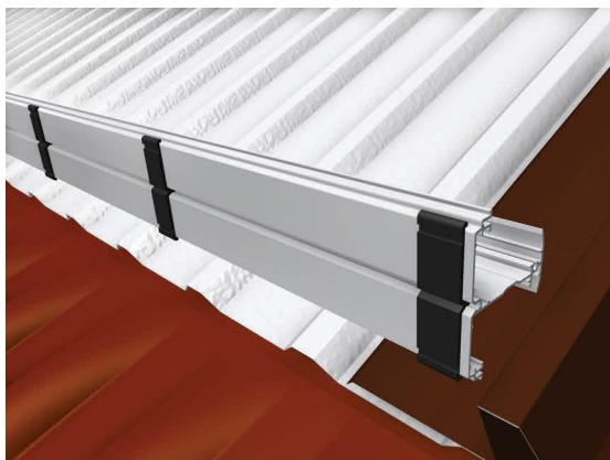
Between the horizontal profiles and the trapezoidal sheet there is corrosion protection rubber which is clamped on the profile in the range of the beat and bolt with it. Also more of the rubber can be used above each other in order to compensate small unevenness.
