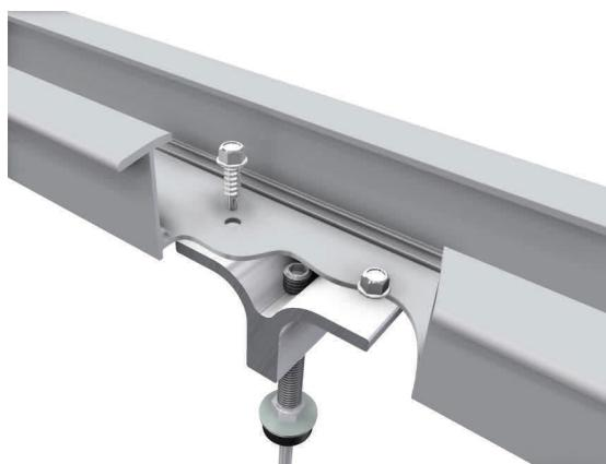
After having adjusted the vertical profiles they are fixed with each 2 drilling screws on the vertical attachment of the solar fastener.
