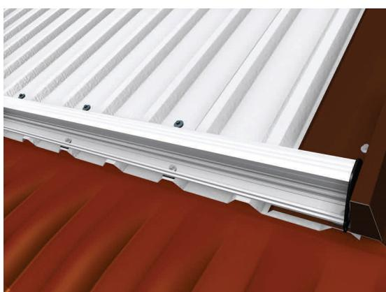
The bolting is done on each other bead (in the edge of each bead) by means of two drilling screws into the drill mark of the horizontal profile.
