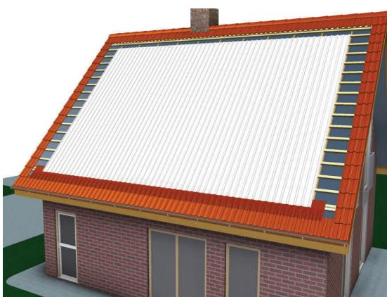
The complete width of the trapezoid roof profile surface must be equal to or at the max. 170mm smaller than the generator width, in order to achieve an optimum connection with the lateral connection plates. The complete height of the surface should be 300mm higher than the generator height, to ensure the sealing by the roof covering in the upper roof connection.
