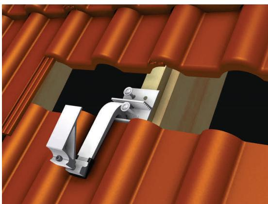
The base plate (70 mm) will be positioned centrally on the rafter and screwed together with two timber bolts (8 x 120 mm) on the rafter. In this connection pay attention to a sufficient wood cross-section and we recommend to pre-drill.
